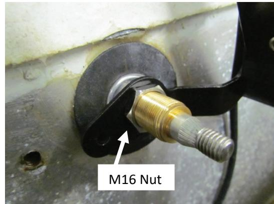
Slide the tapered hole arm head on to the motor shaft
