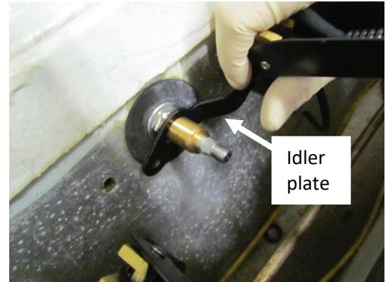
Install the M16 nut over the idler plate and torque to 13Nm - 15Nm
