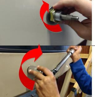
6. Install 7/8" washers and 7/8"-14 Hex Nuts to the outside of the cap, finger tight.
