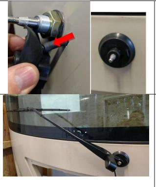
10. Press exposed washer hose onto hose fitting. Slide pivot cap over threaded housing and fit onto hex nut.
