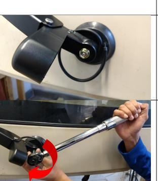
11. Install the wiper arms and blades on the pivot shafts. The wiper arms should park horizontal on the windshield. Install and hand tighten the M8 Hex Nuts onto the pivot shaft threads.
