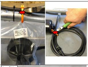
1. Cut Orange zip ties. Leave black zip ties in place, they are needed for the washer system. Open and set aside hardware bag for next step.
