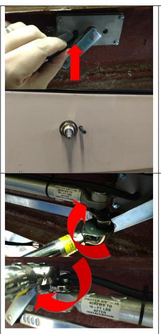
8. Feed the washer tubing through the 3/8" hole. The washer tubing should protrude through the front of the cap.
